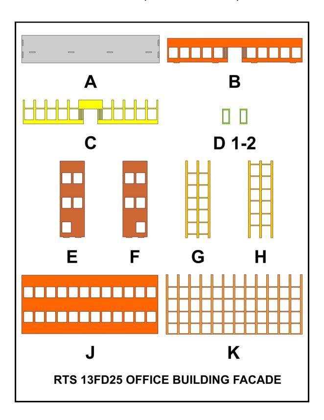
The lower front wall (**B**) and the two side walls (**E**) and (**F**) fit into the foundation (**A**). The higher front wall (**J**) fits against the side walls (**E**) and (**F**). On the walls are window frames, frame (**C**) fits on the lower front wall (**B**); frame (**K**) fits on the higher front wall (**J**) and frames (**G**) and (**H**) fits on the side walls (**E**) and (**F**). Lastly, there are two front doors (**D 1-2**).
